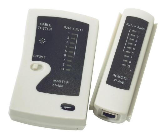
Test Cables & Systems with RJ45 & RJ11 connections. Remote unit allows testing of network runs up to 300m by connection to wall outlets or patch panels. Ideal for verifying the connections on network outlets or individual patch leads. Simple push button operation. LEDs give a clear indication of wiring status Open/short and cross wired wiring test. Connected pin display.
